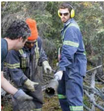
**Figure 7.** Photograph of core barrels used with the Winkie drill for permafrost coring.
