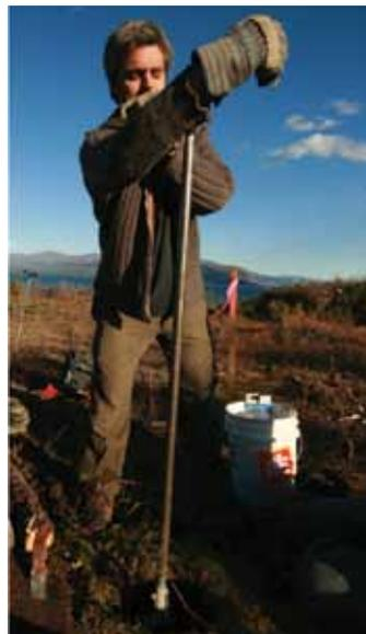
**Figure 10.** Photograph of the hand auger, used for permafrost coring.
