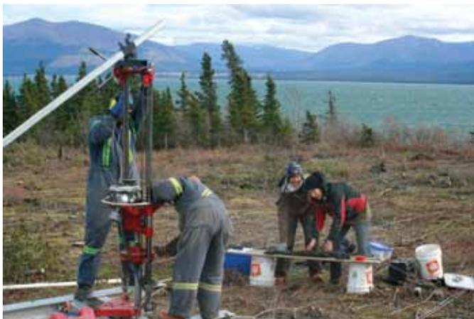
**Figure 5.** Photograph of the Winkie drill, used for permafrost coring.
