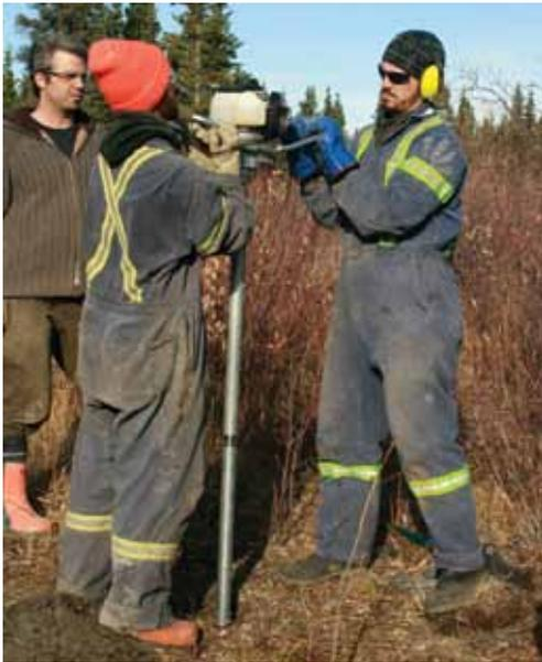
**Figure 8.** Photograph of the CD06 Honda drill, used for permafrost coring.
