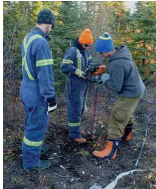
**Figure 9.** Photograph of the auger drill, used for permafrost coring.
