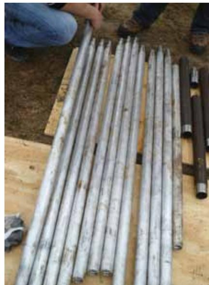
**Figure 6.** Photograph of aluminum rods used with the Winkie drill for permafrost coring.
