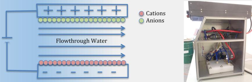
**Purification Stage:** Voltage is induced between electrodes where the impure water stream runs. Cations from the solution migrate to the negative electrode, and anions migrate to the positive electrode. Purified water then exits the system
